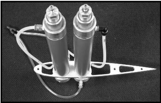
Fig. 16 Integrated wing assembly: pneumatic spars and root rib.
